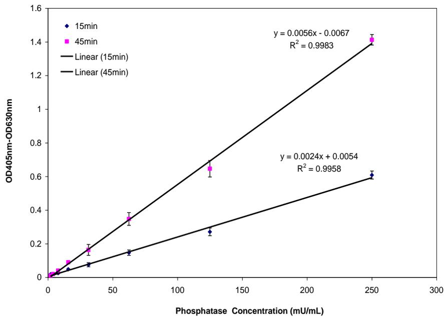
Figure 2. Phosphatase, alkaline from bovine intestinal mucosa was serially diluted in Assay Buffer-alkaline, and its activity was measured with ScienCell™ pNPP Phosphatase Assay after a given time of reaction (15 min and 45 min).
